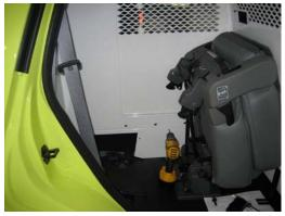
Position floor filler panel to K9 housing, mark holes and pre-drill K9 housing using 1/8" drill bit
